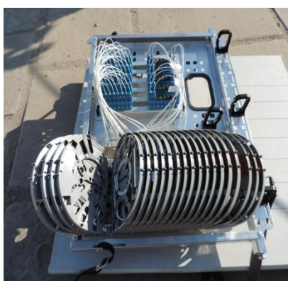
Fig. 14 FDT splicing brackets
